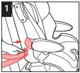
Forward-Facing Use: 22-40 Connect and tighten harness straps prior to installing in vehicle. Place child restraint flush against the back of the vehicle seat forwardfacing in the back seat. The recline position is to be used only to install the . (10.1-18 child restraint flush against
